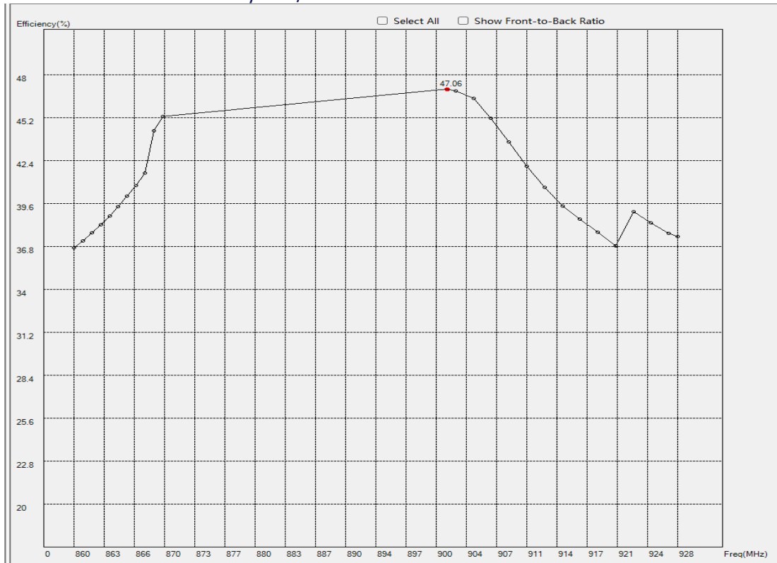
Efficiency (% / Welded on 100*28mm PCB board)
